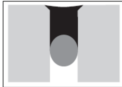
Flush joint design prevents trip hazards and dirt traps
